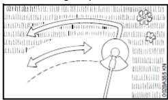
**Brush Knife** To cut dense, matted grass growth or scrub, a brush knife can be used with a chopping effect. Starting at waist height, lower the cutting head on to the growth.
