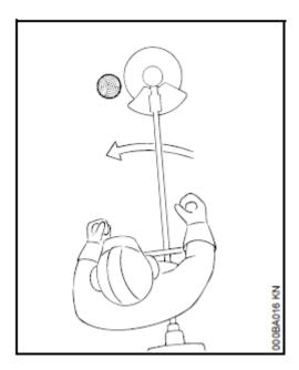
The limit stop should be used to allow the cutting head to be held against the tree being cut. Before starting the cut, accelerate up to full throttle and apply the blade to the right side of the tree.
